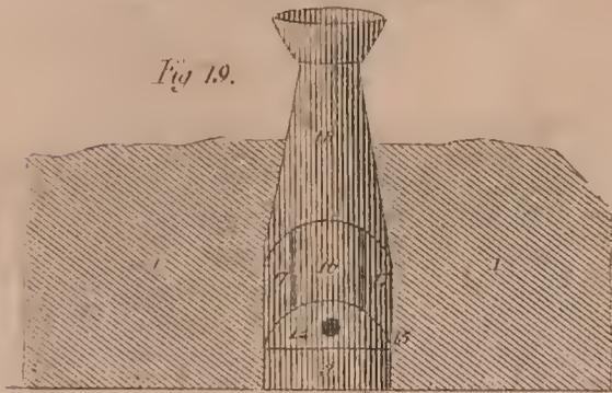
Longitudinal section of the forging furnace.
