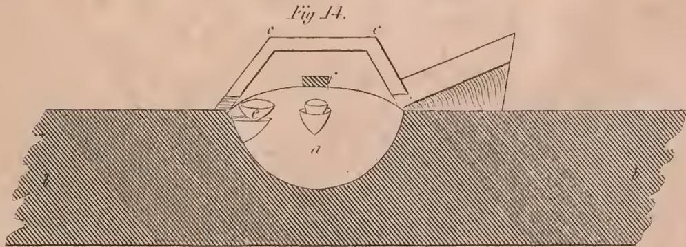
Vertical section of a glass-blower's fire-place.
