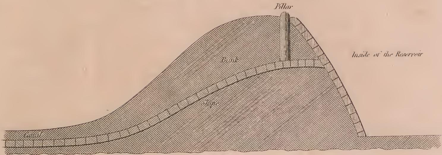
Transverse section of the bank and sluice of an Enay, or Reservoir
